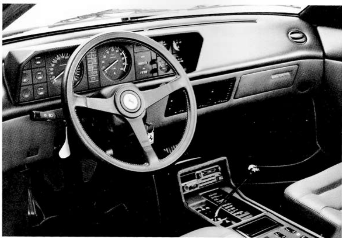
Simple 3.2 Mondial dash with kilometers — therefore, likely European specifications — speedometer. Everything is electronic or electrical now. Ferrari
