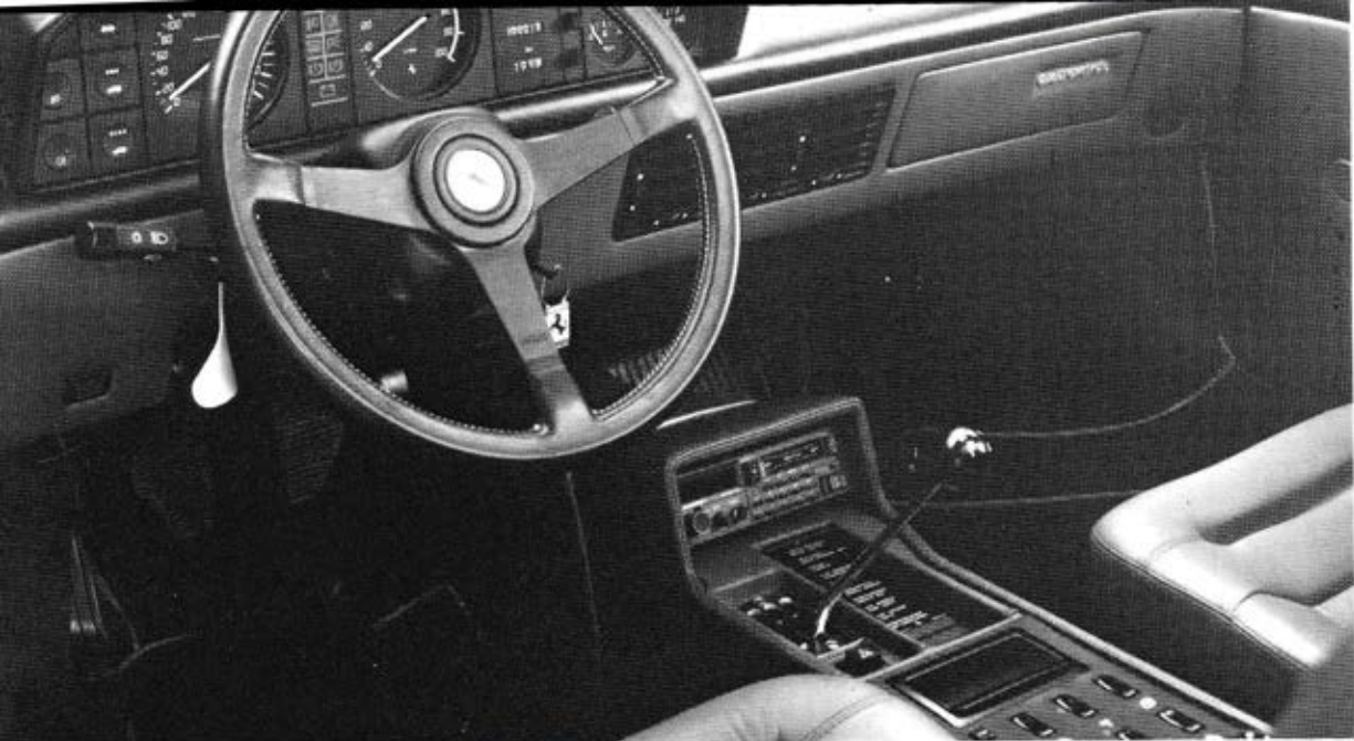
The dashboard of the 3.2 Mondial was redesigned with push-buttons to control many of the features. The center console has a lot of rocker switches and a light warning system. This one has a Blaupunkt radio, but there is no "official" Ferrari radio.
