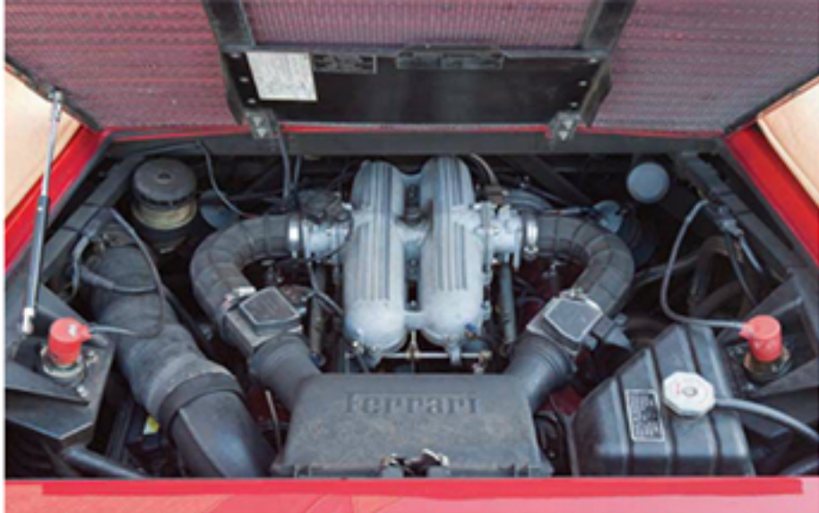
By aligning the Mondial T's 300-hp, 3.4-liter engine longitudinally in the chassis—a first for a mid-engined V-8 Ferrari—engineers were able to mount it five inches lower, improving handling.
