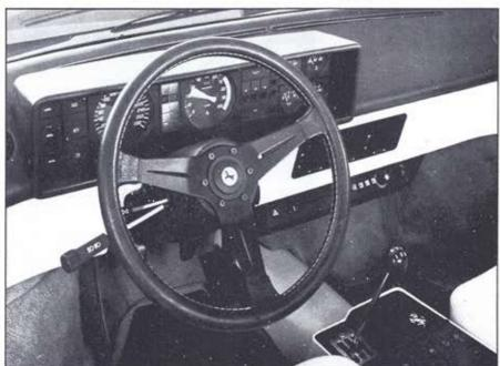
Above: Panel of warning lamps behind radio informs on state of (from driver's right to left) engine temperature, brake hydraulics, bonnets open, transmission oil level, engine oil, screen washer fluid, service due, stop lamps, parking lamps, and air conditioning
